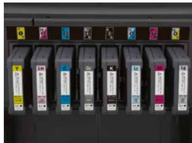
Sub Tanks View behind the dismantled cover:
