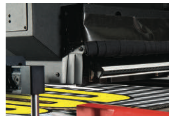
Shuttle safety sensors prevent printheads from touching the substrate. The ionizer bar avoids electro static loads. Both are located on the shuttle.
