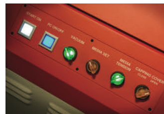
An automatic vacuum system delivers an equal vacuum throughout the whole printing process.
